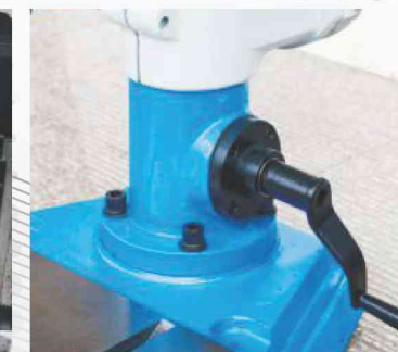
SPINDLE HEAD RISE/ DOWN BY HANDLE
